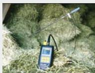
The set consists of GMH 3830 with preset material selection (Sort) and a rugged integrated probe (15) with integrated temperature sensor.
